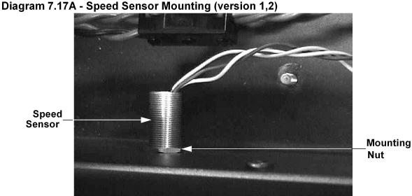
Remove the mounting nut that secures the speed sensor assembly to the frame. Thread the speed sensor out of the frame.
