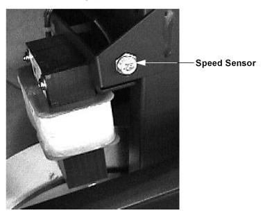
12. Remove the mounting nut that secures the speed sensor assembly to the frame. Thread the speed sensor out of the frame.
